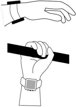
**Figure 1:** Smartwatch concept with two displays – one on each side of the user’s arm. Depending on the arm’s orientation, the content can be shifted between the displays: when doing pull-ups for example, the inner display can still be seen while the outer one is not in the user’s field of view.
