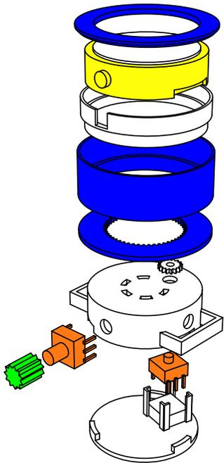
**Figure 1:** Exploded view of the self-built smartwatch housing with the Moto360 (yellow) and the mechanical components: crown (green), rotatable bezel (blue) and the corresponding rotary encoders (orange).
