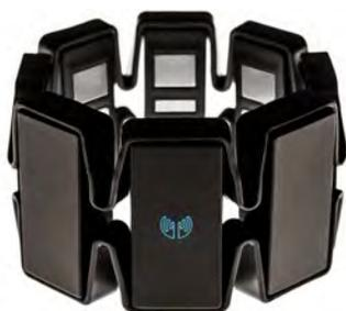
Figure 3: Electromyography armband by Thalmic Labs
